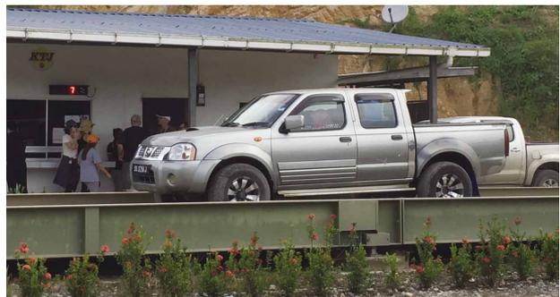
The Kemajuan Tanah Julur Collection Center opened in 2017. They weigh the delivery trucks before and after unloading the fresh fruit to calculate the actual weight of the fruit. They apply a daily exchange rate for the purchase. The center enables them to transfer FFB weighed fruit collectively instead of being sold separately to mills. Unfortunately, the center does not yet have RSPO certification.
